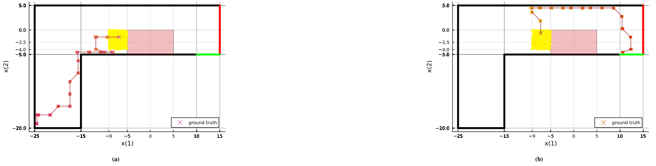
Fig. 6: Plot of one of the trials of the execution of the actions from planning in Lidar Roomba problem. Illustration of departing from the unsafe region problem in Lagrangian based methods. The yellow rectangle represents 500 particles of b_0 sampled from a uniform distribution, the pink rectangle is the unsafe region to avoid. The green line is the exit area and the red line is the stairs. On both figures we plotted the ground truth robot positions and the beliefs that transit from yellow to red as time indexes progress; (a) CPFT departs as far as possible from the unsafe region. (b) Our method behaves as expected: the agent goes to the green area while avoiding the unsafe region.
