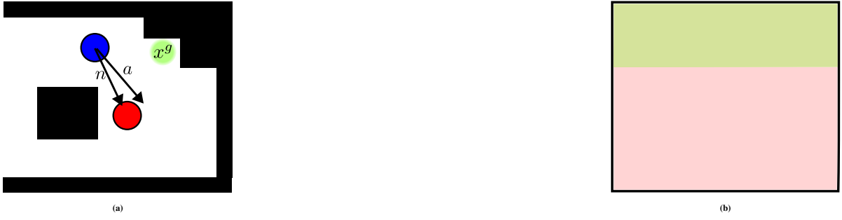
Fig. 7: (a) Conceptual visualization of the PushBox2D problem. The agent is the blue circle. The puck is the red circle. The goal is the green circle. (b) The observation noise intensity map. Light green color denotes the lower noise intensity.
