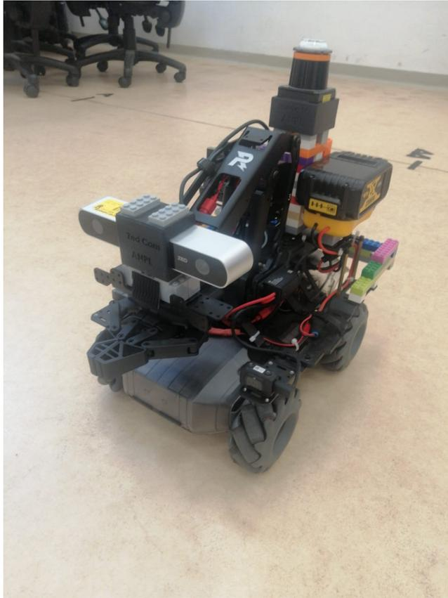
**Figure 4.10:** Robomaster S1 robot, equipped with a ZED camera
